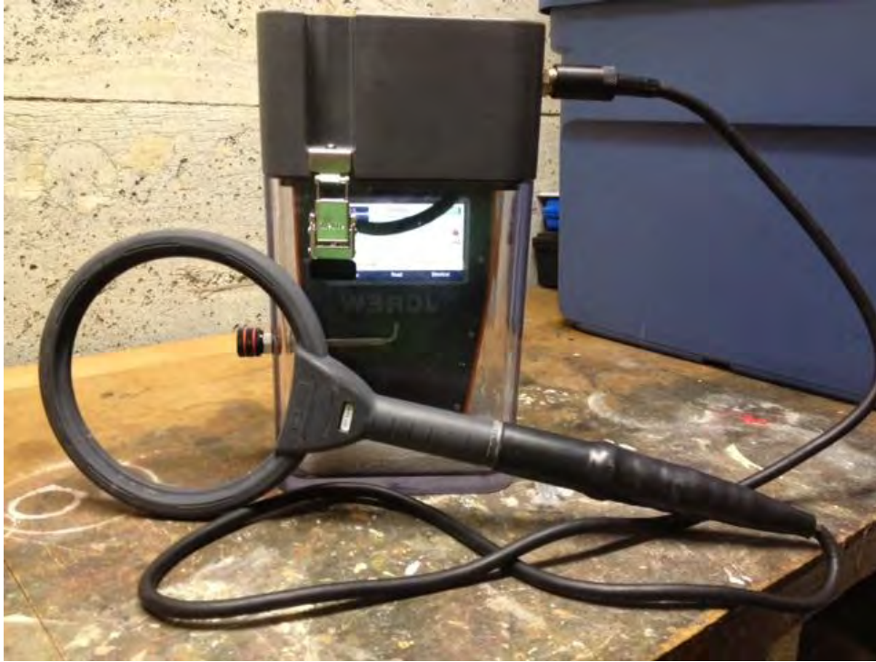
Figure 6. Biomark HPR Plus PIT tag reader contained in a custom Preveco Subsea dive housing.
