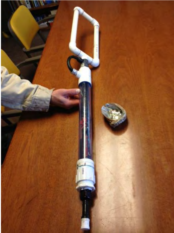
Figure 7. Underwater PIT tag reader developed and constructed by NOAA biologists.
