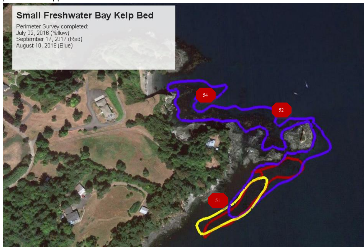
Figure 5. The map of the small kelp bed at Freshwater Bay based on the field recorded GPS readings taken August 10, 2018 (Google Earth map). The purple/blue line depicts the extent of the kelp bed in 2018, the red line in 2017 and the yellow line in 2016. The red number boxes - waypoints - indicate where depth and temperature measurements were taken.
